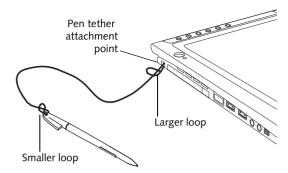
Figure 2-2. Installing a Pen Tether
